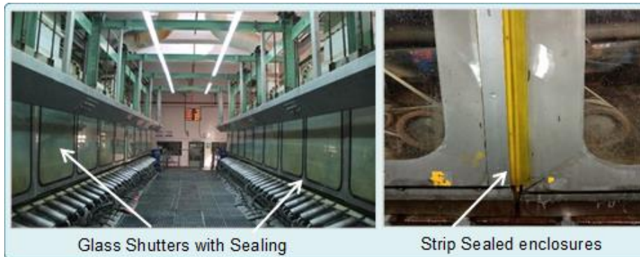
Figure 4 – Spinning Machine with Closed-loop Technologies
